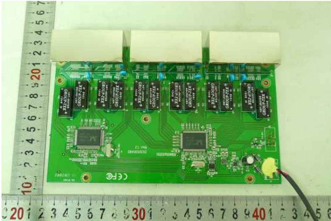
Figure 9. Main board PCB components side view
