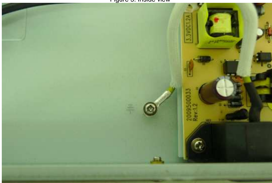
Figure 6. Protective bonding terminal
